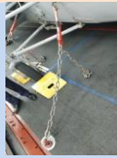
Deck Mooring Device
